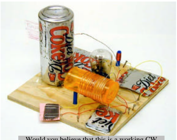
Would you believe that this is a working CW transmitter using no electronic parts?
